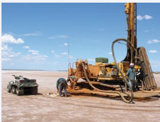
Aircore Drilling, Lake Way, WA – February 2007
